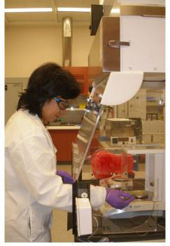
Weighing nanomaterials in a HEPA-filtered balance enclosure
